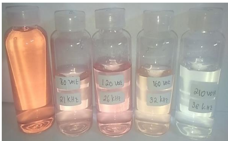
Figure 12. The results of degradation of the Congo Red solution with variations in input stress
